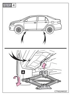
Turn the tire jack portion "A" by hand until the notch of the jack is in contact with the jack point.
