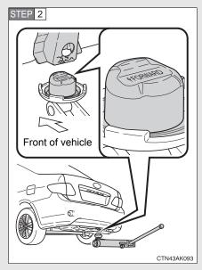
Set the jack attachment on the floor jack with the "FOR-WARD" facing towards the front of the vehicle, and place the jack.
