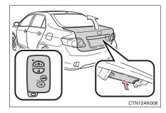
Press the button to unlock the trunk.
