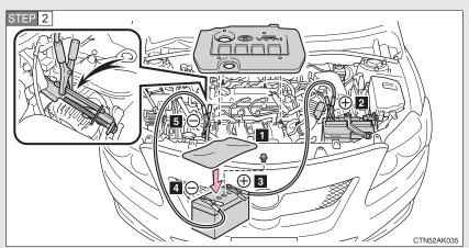
Connecting the jumper cables
