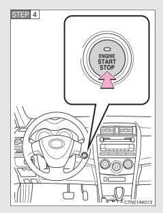
Press the "ENGINE START STOP" switch.
