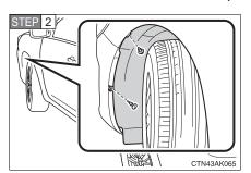
Remove the fender liner clips.
