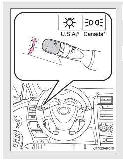
The side marker, parking, tail, license plate and instrument panel lights turn on.
