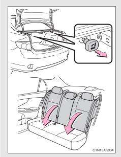
Pull the seatback lever in the trunk for the seatback you wish to fold down.
