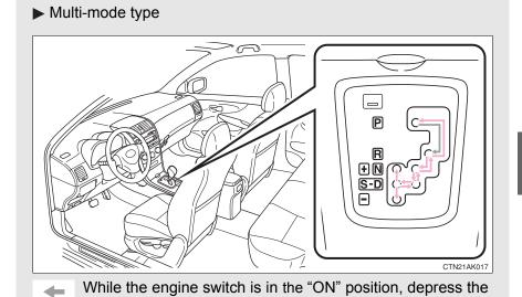
brake pedal and move the shift lever.
