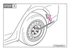
Slightly loosen the wheel nuts (one turn).
