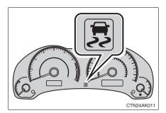
If the vehicle is in danger of slipping or the front wheels spin, the indicator flashes to indicate that VSC/TRAC have been engaged.
