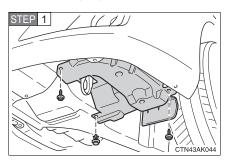
Remove the fender liner bolts and clip.
