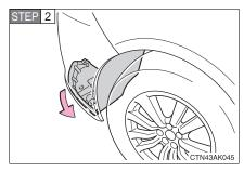
Partly remove the fender liner.
