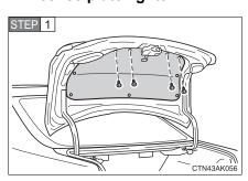
Open the trunk lid and remove the trunk panel cover clips.
