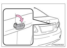
Turn the mechanical key clockwise to open.
