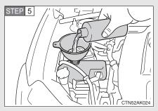
Add engine coolant if necessary.
